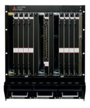
The Casa Systems C10G is a new class of cable edge device that combines a third generation DOCSIS 3.0 CMTS and an MPEG video Edge-QAM in a high density, high availability 12RU platform.
